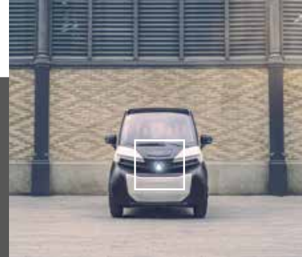
Central light (low and high beam) and side lights (position and DRL)
